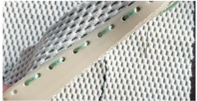
► Fig. 48 Double thread stitch
