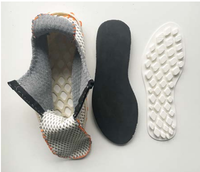
► Fig. 51-52 Shoe, midsole (black) and outsole (white)
