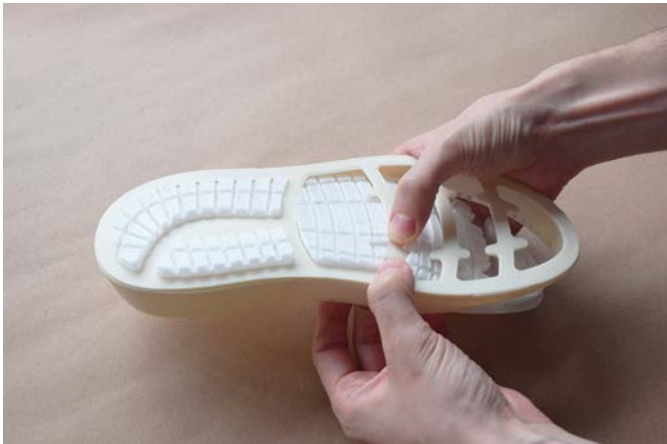
► Fig. 55 Interlocking system between outsole and sole
