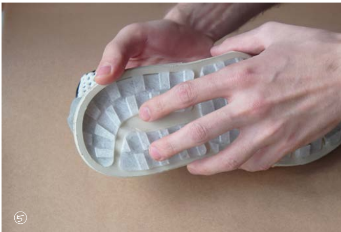
► Fig. 62 Outsole insertion
