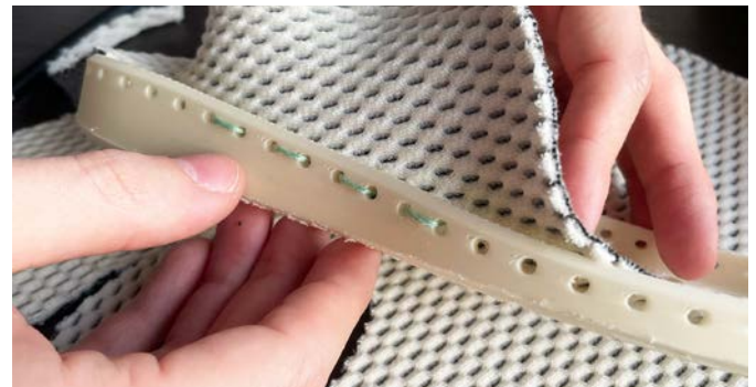
► Fig. 49 Single thread stitch
