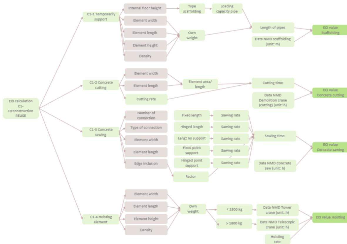
Figure E.13 Process tree - ECI value Reuse deconstruction (Own figure)
