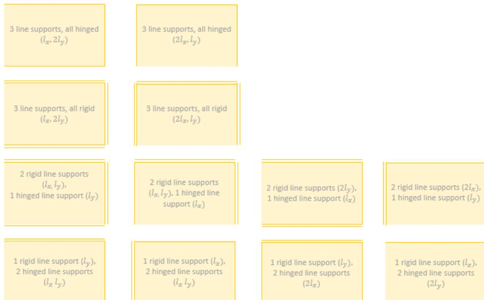
Figure D.9 Options for three-sided supported floor elements (Own figure)
