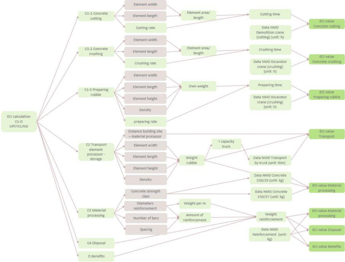
Figure E.16 Process tree - ECI Upcycling Demolition, Transport, Post-processing, Disposal, Benefits (Own figure)
