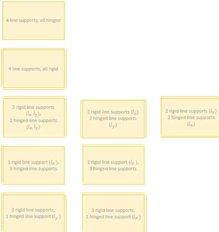
Figure D.10 Options for four-sided supported floor elements (Own figure)
