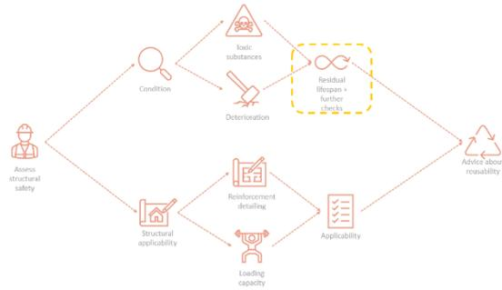
The complete process of analysing the condition of a structural element is visualized in the process tree in [Figure E.2](#).
