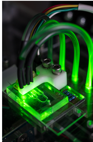
Figure 2.2: An example of a microfluidic device mimicking blood vessels as sourced from Georgia Institute of Technology [26]
