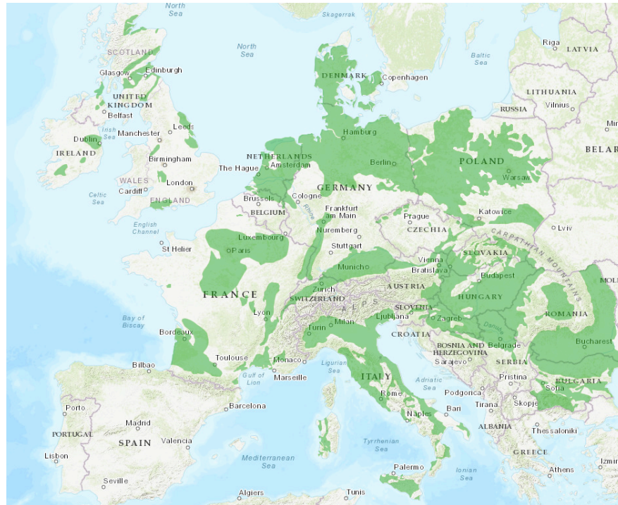
Figure 5.2: A map of Europe where the green areas display regions with economic hydrothermal potential. In short, this means that an area's subsurface contains sufficient geothermal energy, combined with subsurface characteristics that make it suitable for economic exploitation. Note: Portugal has not been included in the study resulting in this data set (source: Europa-Universität Flensburg et al., 2021).
