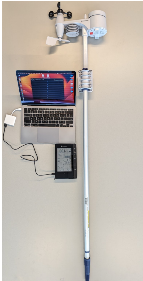
Figure 6.2: Instruments used to measure wind direction and magnitude: weather station, support pole, USB radio receiver, and a laptop.
