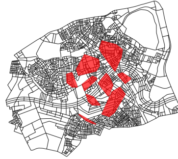
(b) Intrusion-based clusters with a high density categorisation at 50 minutes of a simulation with 400 aircraft.
