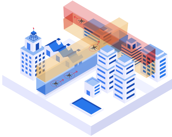
Figure 2.2: Constrained airspace intersection example. Note how the blue and red cruise layers are vertically separated and contain a turn (yellow) layer in between. Note that this pattern is stacked until the top of airspace. The red circles and arrows signify the protected zone and current direction of travel of the drones, respectively.
