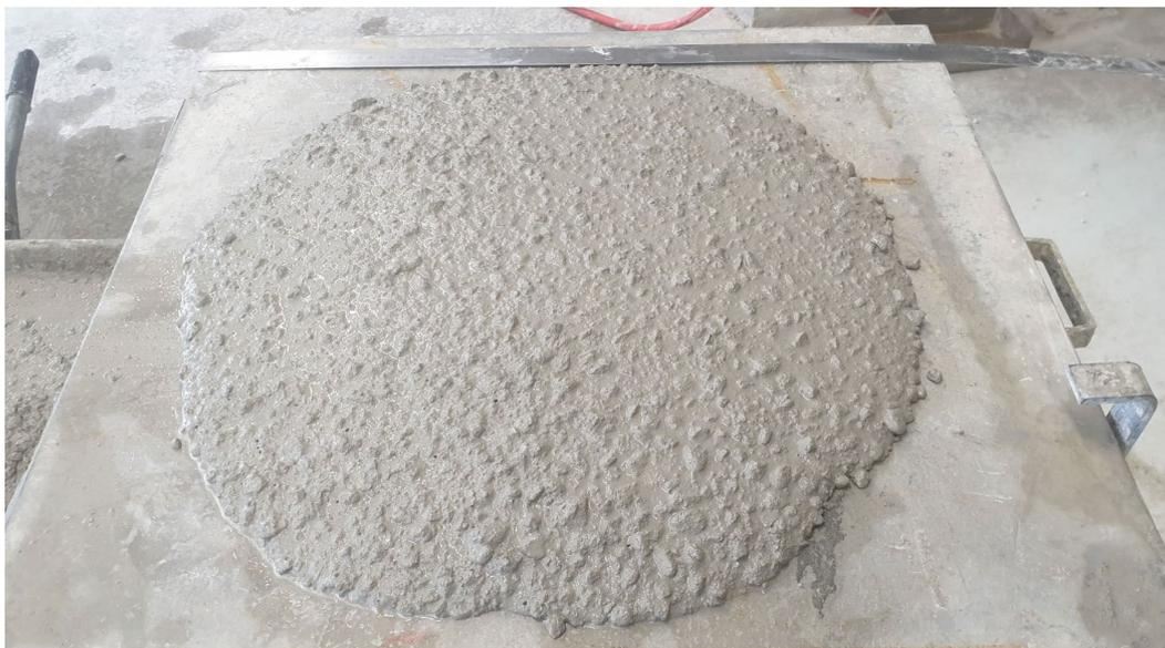
Figure 3.7: Consistency of concrete made with 100% RCA.
