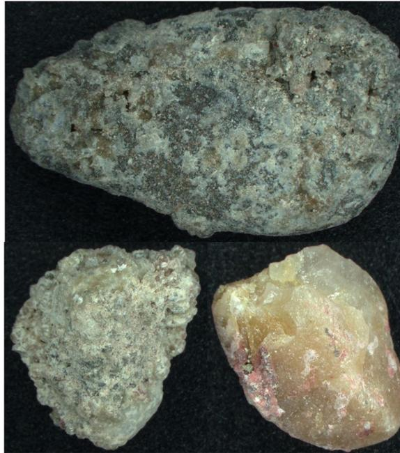
Figure 2.1: Different fractions of RCA
