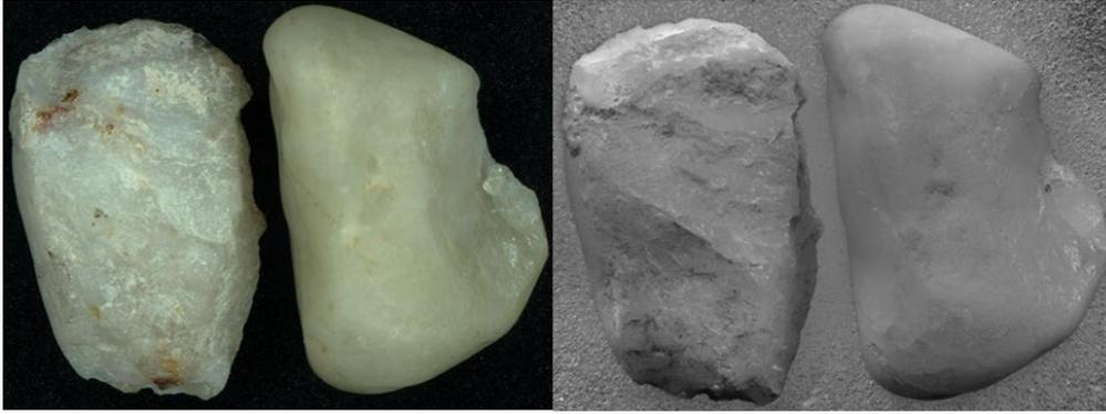
Figure 5.2: Microscopic and optical shadow effect mode image of RCA type R<sup>2</sup>(Left) vs. NCA (right).
