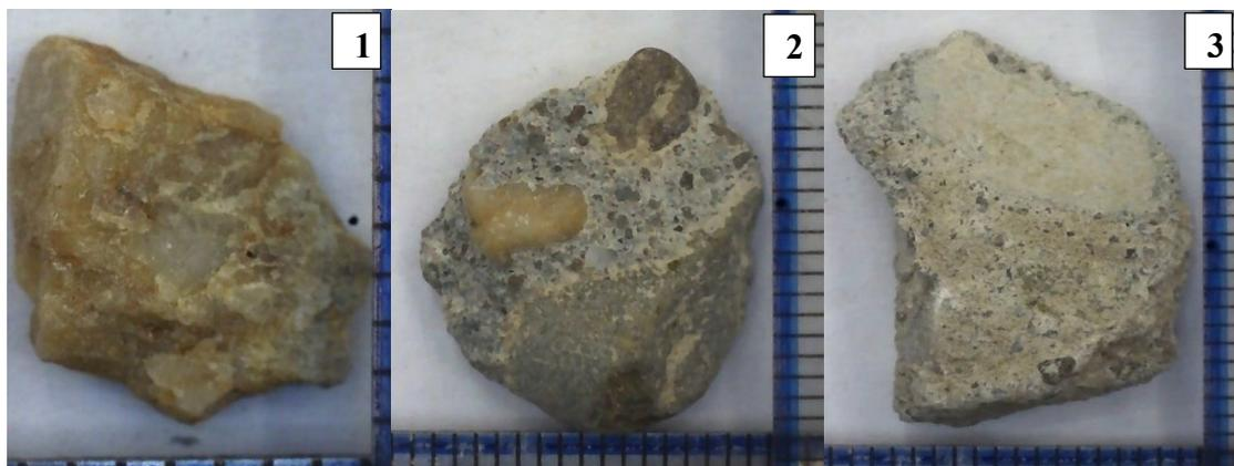
Figure 3.1: Different types of RCA fractions.
