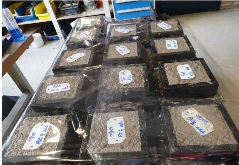
Figure 3.2: Concrete casted in moulds
