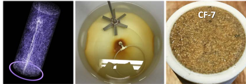
Figure 5-15: Left: CT scan image of fracture along the core, Middle: Rust formation in injection bucket, Right: Injection face of the core after exp. CF-7
