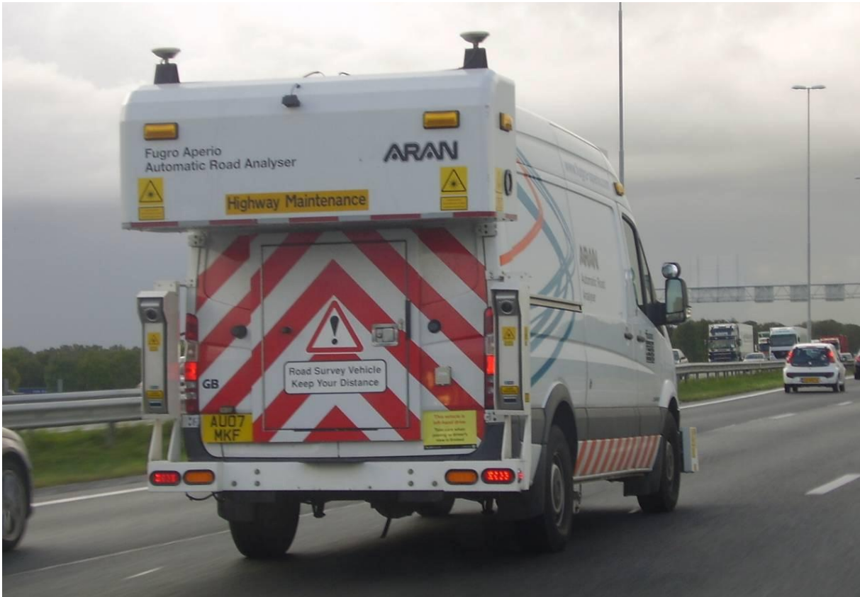
Figure 23, ARAN vehicle measuring road conditions (Blanken, 2013).
