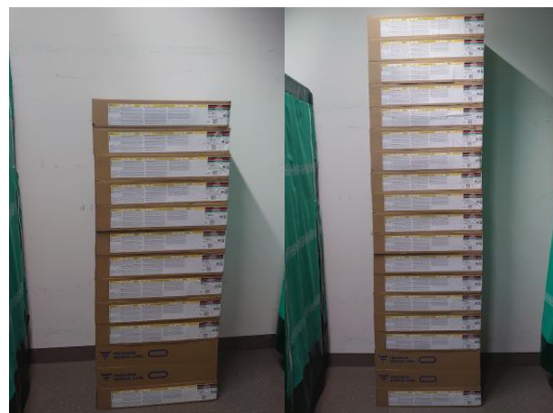
Figure 68: 12 and 18 full boxes stacked on top of test box
