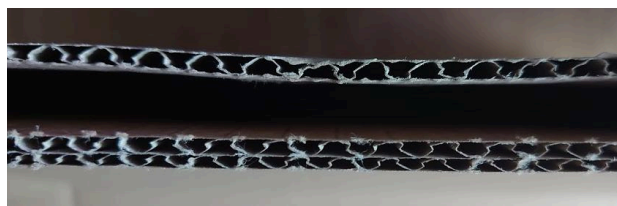
Figure 64: Profiles of the top and bottom sheets
