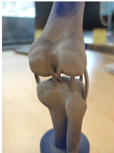
Figure 13: Posterior view of the 3D printed design of the knee joint after applying the black-dot speckle pattern for DIC testing.
