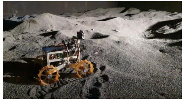
**Figure 15.9:** Small rover prototype testing in the lunar environment test bed at the University of Luxembourg [95].
