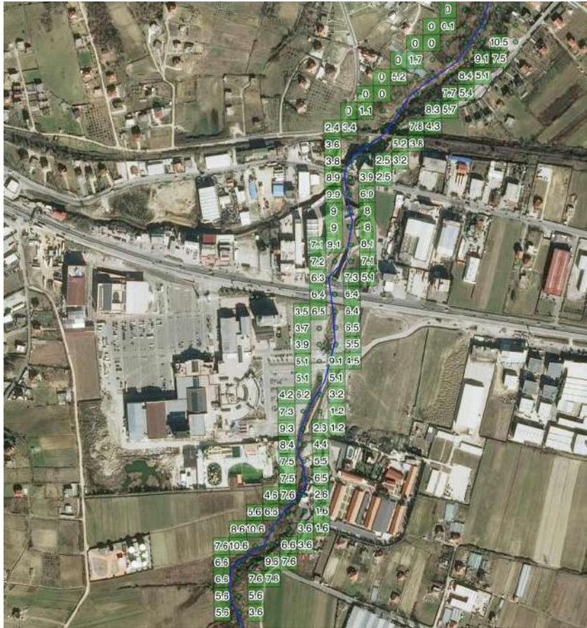
Figure 27: Height of the water retaining structures that protect the City Park area. The dredging depth and the addendum are already included in the calculation.
