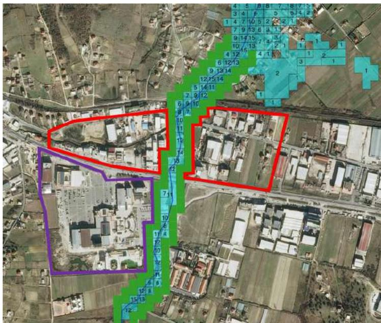
Figure 25: Location of the water retaining structures (green) and water depth in the City Park area. The commercial and industrial area of the City Park are marked in purple and red, respectively.
