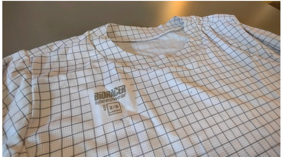
Figure 2. Custom made research garments in the standard confection sizes. The custom print consists of a 1 \times 1 cm grid of lines that aid in 3D scanning and measuring of stretch.
