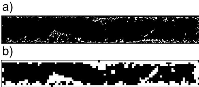
Fig. 5. (a) Segmented porosity cross-section on the  $xy$  plane, where pores are highlighted in white; (b) same cross-section after max-filtering with a cubic element of 15 voxels side, corresponding to approximately 1.5 times the fibre diameter.
