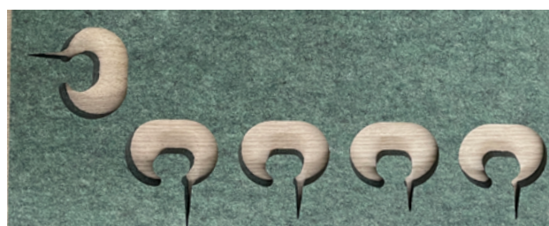
Figure 92: Geometry 5 with different notch sizes
