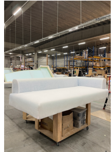
Figure 8: Dacron layer applied
