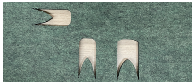
Figure 93: Redesign of anchor, different sizes to test stiffness
