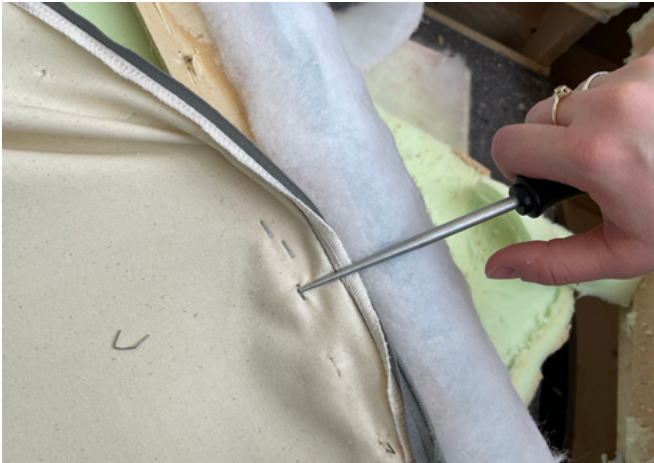
Figure 23: Prying staples loose from fabric cover with awl
