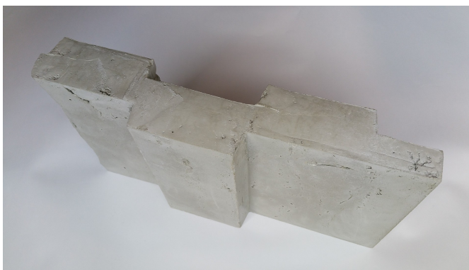
Figure 4.3: The mortar filling after demoulding
