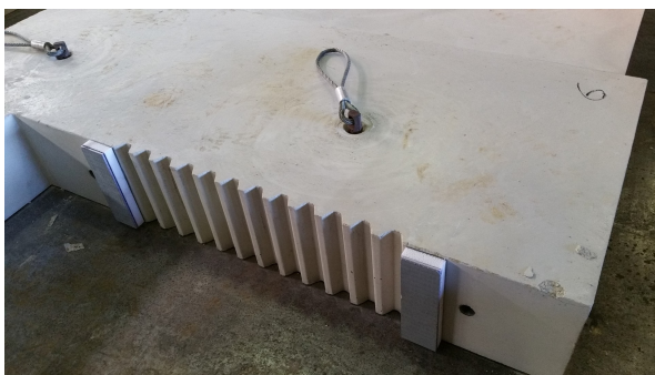
Figure 4.9: Spacers between L-elements
