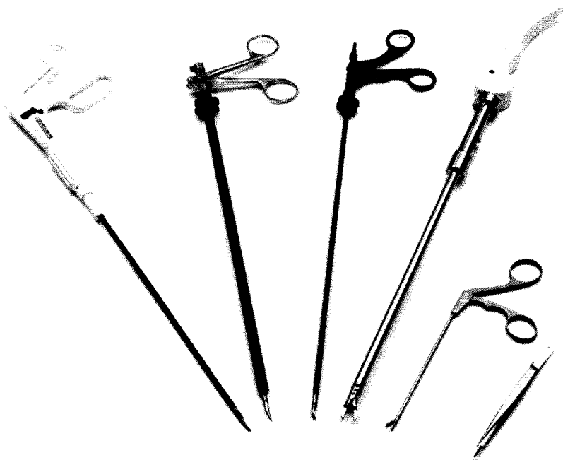
Figure 2. The instruments tested (from left to right); 5 mm disposable dissector, 10 mm reusable dissector, 5 mm reusable dissector, Wilmer® dissector, orthopaedic dissector, tweezers.
