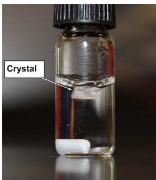
Figure 2.9: Single crystal of paracetamol probably formed at the air-liquid interface.
