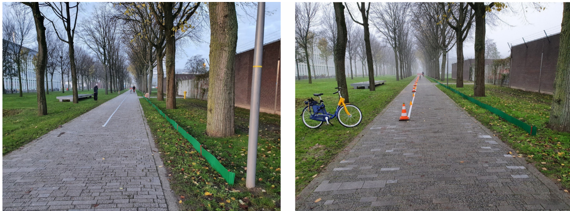
Fig. 3. Two methods used to attach the white band to pavement: first measurement day left and second measurement day right.
