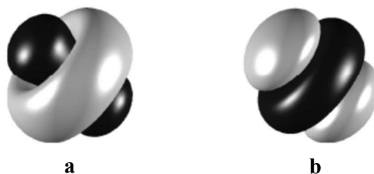
Figure 13. Two types of three-dimensional steerable filter kernels for detection of image structures. Positive kernel factors are depicted in black and negative kernel factors are depicted in grey. a. The kernel for curve detection. b. The kernel for surface detection. Figure adapted from [53].
