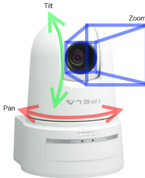
Figure 1.2: The pan-tilt-zoom camera can pan horizontal, tilt vertical and zoom its optical lens.
