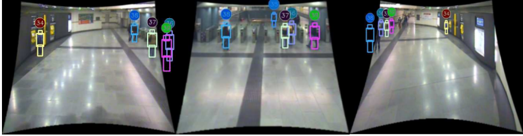
Figure 2.13: The targets are identified in three different cameras and labeled with the same number and color. The system contains a shared mental model. From Yao and Odobez, 2008.
