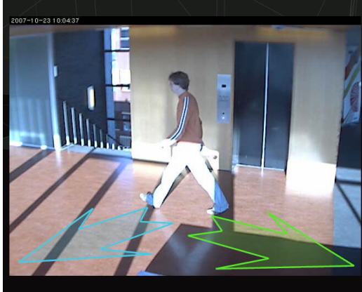
Figure 2.6: The arrows shown in the image correspond to neighboring cameras. The user can click the arrow to fly to that camera.
