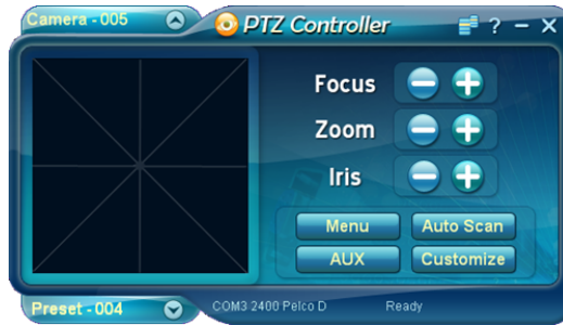
Figure 2.12: A virtual PTZ joystick. Zooming is implemented as simple buttons on the right. The mouse is controlled within the left square. From http://serialporttool.com .
