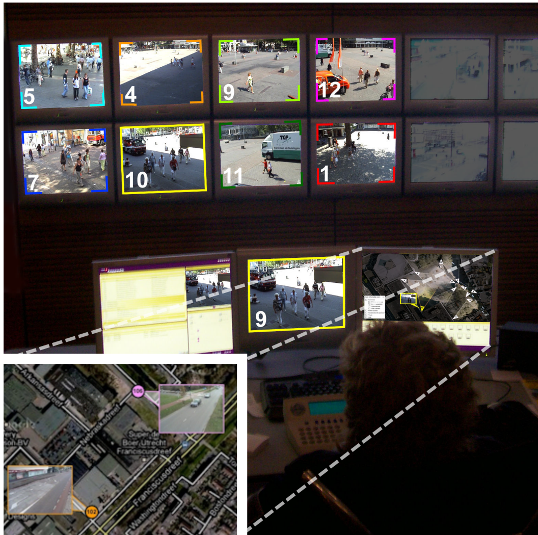
Figure 2.24: An early version of the TNO Slim Toezicht project in association with S&T Vision. All video screens are color coded. The color codes are used to associate the images with points on the screen. Bottom left: A low resolution image of the final version that is currently active in Utrecht. The camera cones show the view direction of the PTZ camera.
