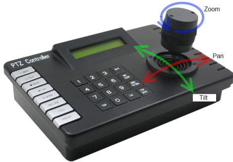
Figure 2.11: A common PTZ joystick controller with extra function buttons that can pick the active camera to be controlled and set camera to preset orientations. From http://worldeyecam.com
