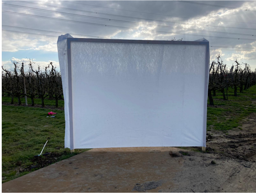
FIGURE 3.10: The setup of the screen placed above a steel road plate on top of bare soil.
