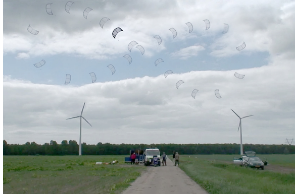
Figure 2.1: Crosswind figure eight trajectory flown using the Laddermill prototype kite power plant. The wind vector points along the road towards the horizon.
