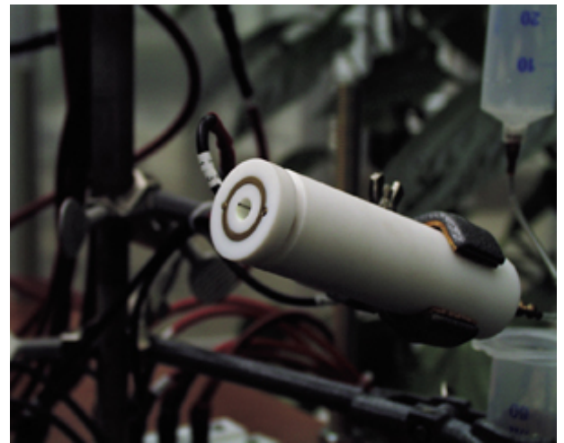
The electrospraying technique given shape in the form of a nozzle as used by Kees Geerse in his greenhouse tests. The nozzle was designed by Charles Marijnissen, the 80-year old uncle of Dr. Ir. Jan Marijnissen, and was made at the faculty workshop.
