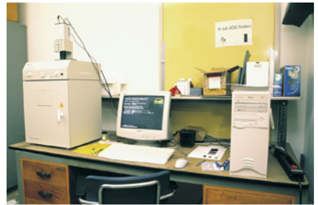
Test set-up for the analysis of the sprayed leaves. It consists of a microcomputer (on the right) and a dark chamber (on the left) carrying a very sensitive camera.
