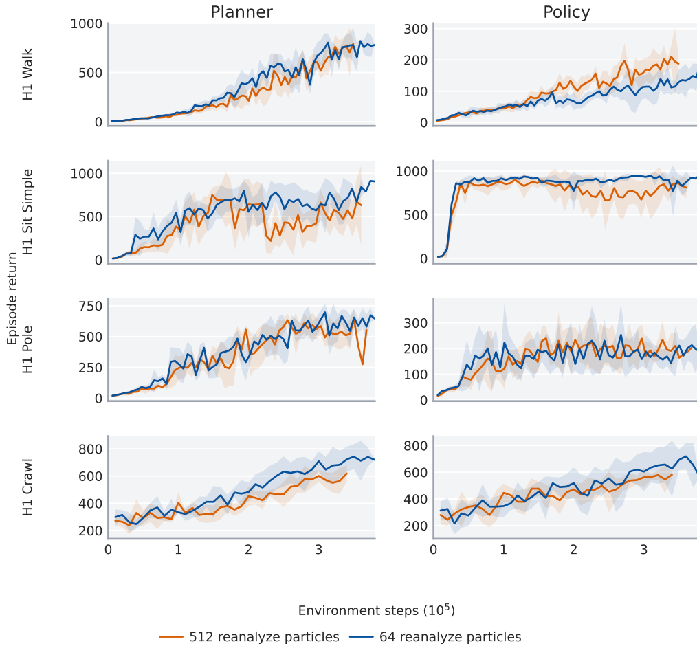
Figure A.5: Reduced reanalyze compute does not degrade performance much. The per-task planner and policy learning curves show that training BMPC with 8x fewer reanalyze particles does not noticeably degrade performance on four HumanoidBench tasks with 61 action dimensions. The accompanying compact aggregate summarizes the normalized planner performance over the same four tasks. Shaded regions denote 95% confidence intervals over available seeds.
