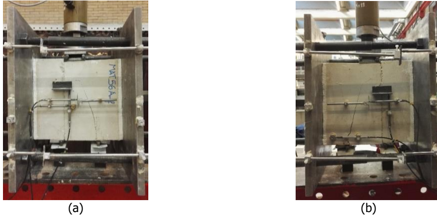
Figure 48 – Typical observed cracks including vertical crack in the joint and diagonal crack in the unit (specimen TUD_MAT-56A-f): (a) front side; (b) back side.
