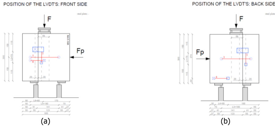
Figure 47 – Arrangement of the LVDT's: (a) measuring system arrangement 1; (b) measuring system arrangement 2.
