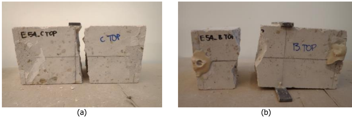
Figure 8 – Crack pattern for sawn-cut specimens (200x100x100-mm): (a) symmetric crack pattern; (b) asymmetric crack pattern.
