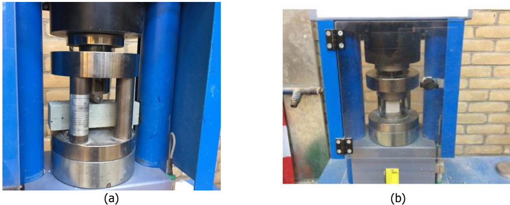
Figure 3 – Test on masonry mortar specimens: (a) three-point bending test; (b) compression test.
