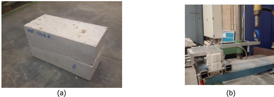
Figure 40 – Bond wrench tests: (a) couplets adopted for the test; (b) improved bond wrench set-up.
