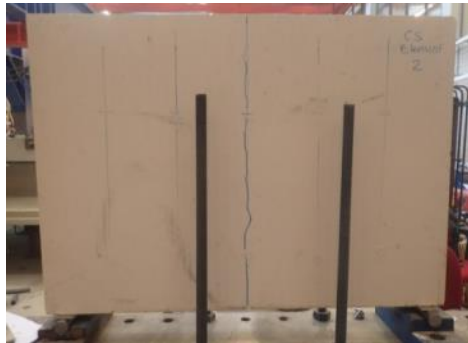
Figure 10 – Symmetric crack pattern for full-scale calcium silicate element subjected to three point in-plane bending (897x643x100-mm).
