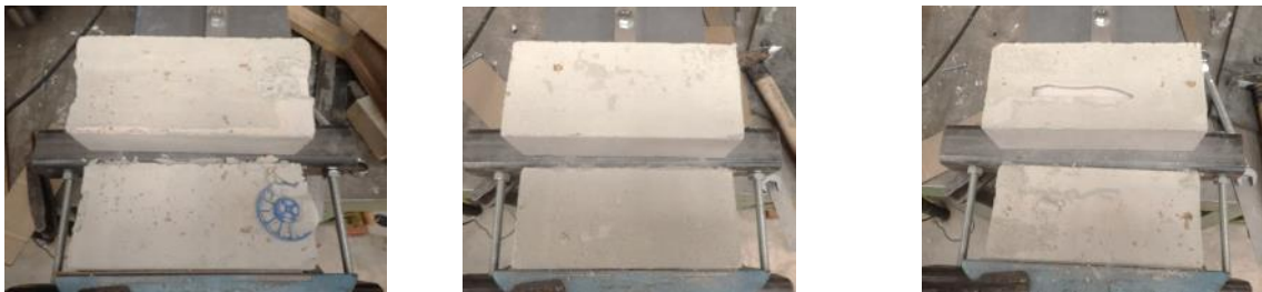
Figure 43 - Observed failure mechanisms: (a) type B for sample type I (with hole); (b) type A and, (c) type B for sample type II (without hole).
