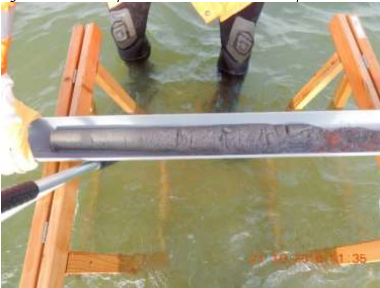
Figure 0-9 Sampled sediment core with piston sampler
