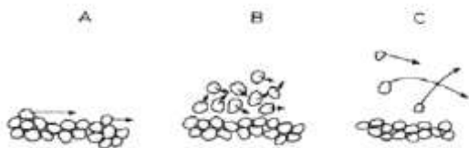
Figure 2-15 Modes of sediment transport. A: bed load at low shear stress, B: sheet flow at higher shear stress, C: suspended load (source: (Fredsoe & Deigaard, 1992))
