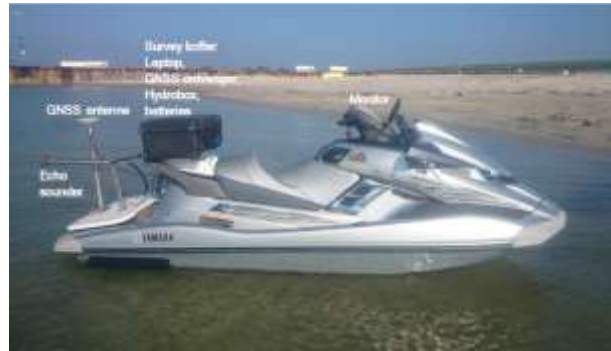
Figure 3-9 Right: Jet ski with acoustic measuring devices as used in the measurement campaigns
