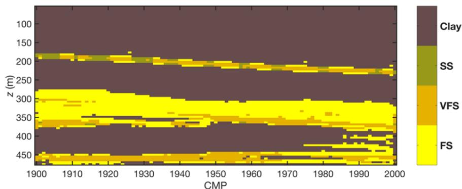
**Figure 5** Starting model in terms of lithologies.
