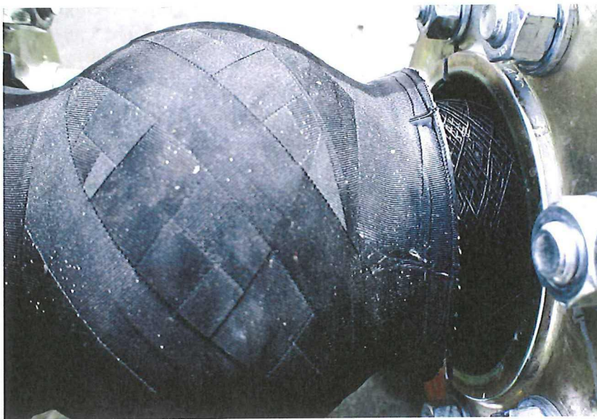
FIGURE 4.9: RUPTURED OUTER RUBBER IN SINGLE-LAYERED PROTOTYPE
