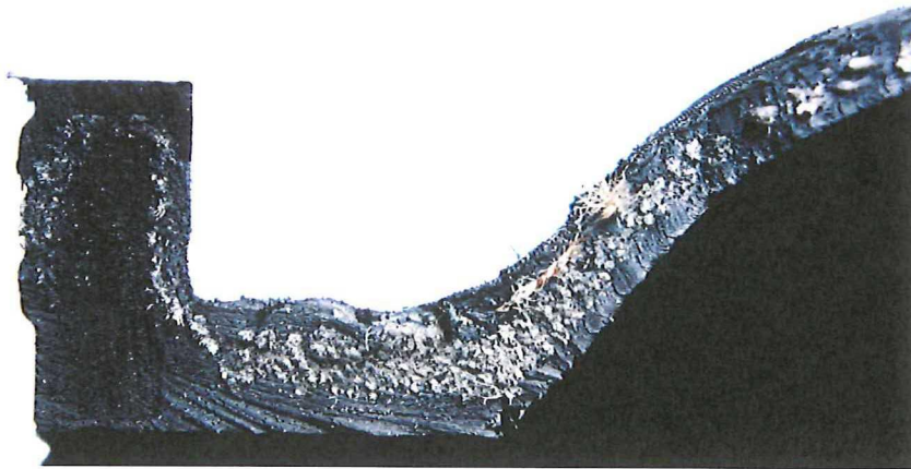
FIGURE 6.2: FIBRE DISTRIBUTION NEAR THE FLANGES OF AN EXPANSION JOINT
