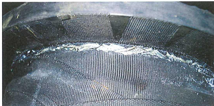
FIGURE 6.1: RUBBER TEARING FAILURE[26]
