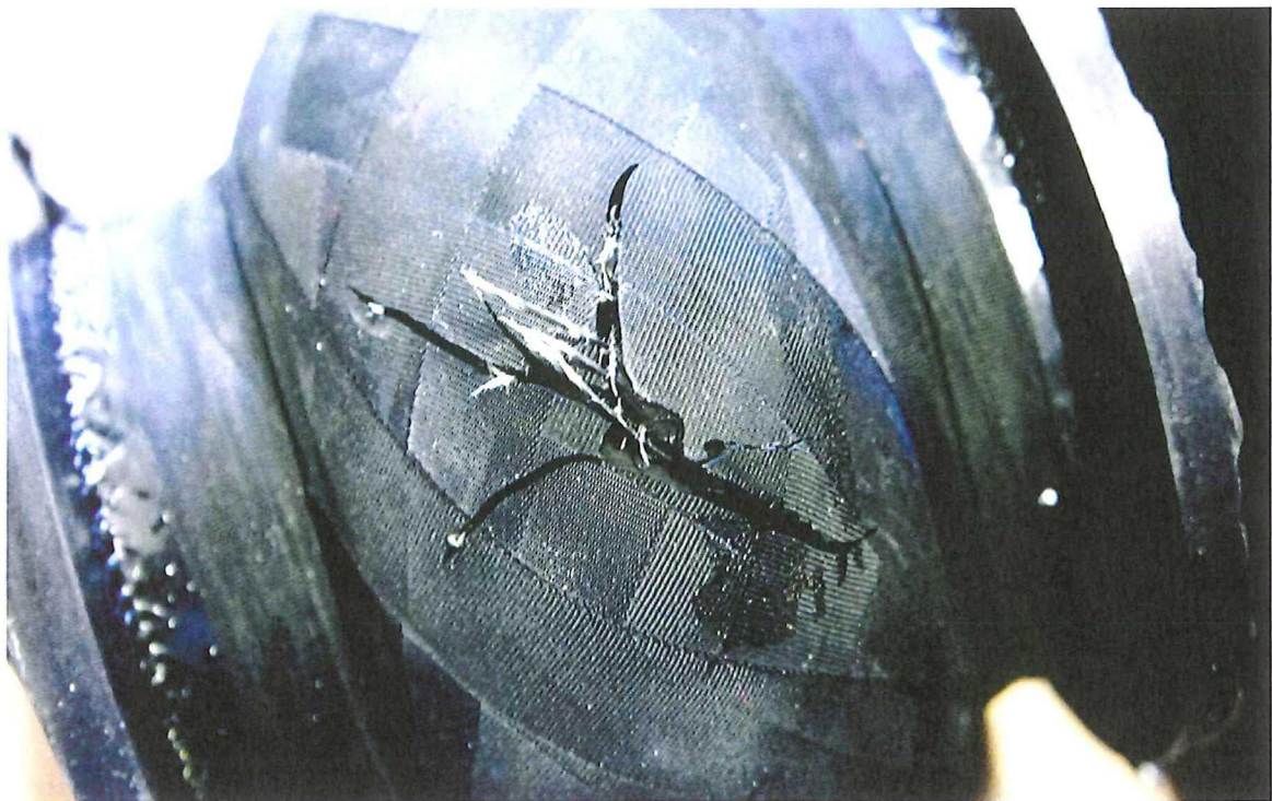
FIGURE 6.3: FIBRE BURST FAILURE
