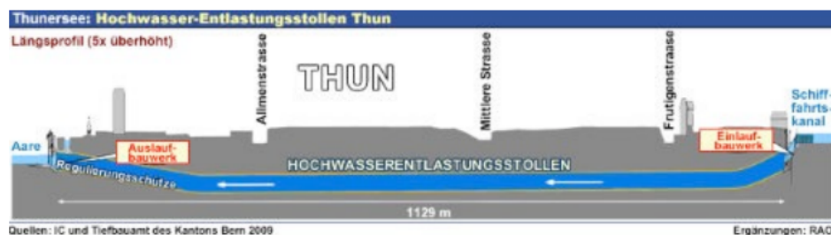
Figure D.8: Flood bypass tunnel Thun (Autor & Bruderer, 2020)
