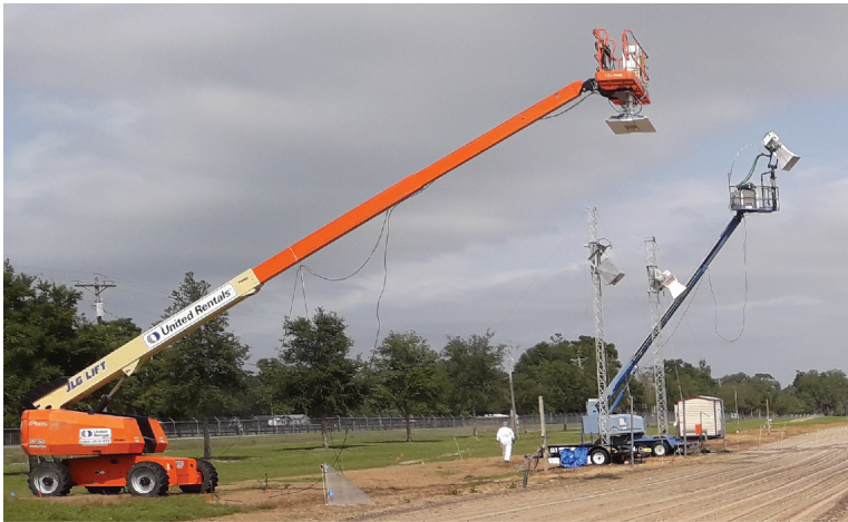
Figure 2.3: Scatterometers in Florida 2018 before sowing. The UF-LARS system is mounted to the blue crane (right).
