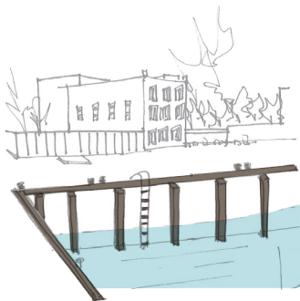
Breakwater- wooden posts - anchors
