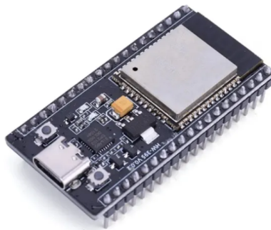
Figure 3.2: Image of ESP32-DEV-38P [28]
