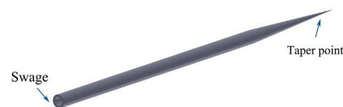
Fig. 1. Schematic illustration of straight stainless steel tapered needle.
