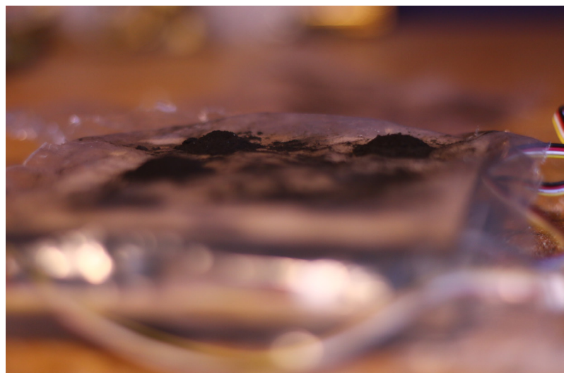
Figure 48 Testing formation of tactile bumps using iron filings
