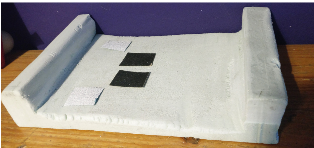
Figure 50 A foam mockup with sanding paper tiles, of different grit sizes stuck.
