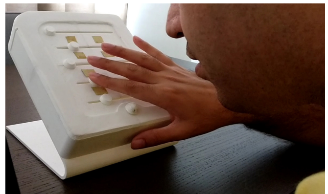
Figure 70 3D printed form prototype presented to a blind programmer, for tactile perception of the product.
