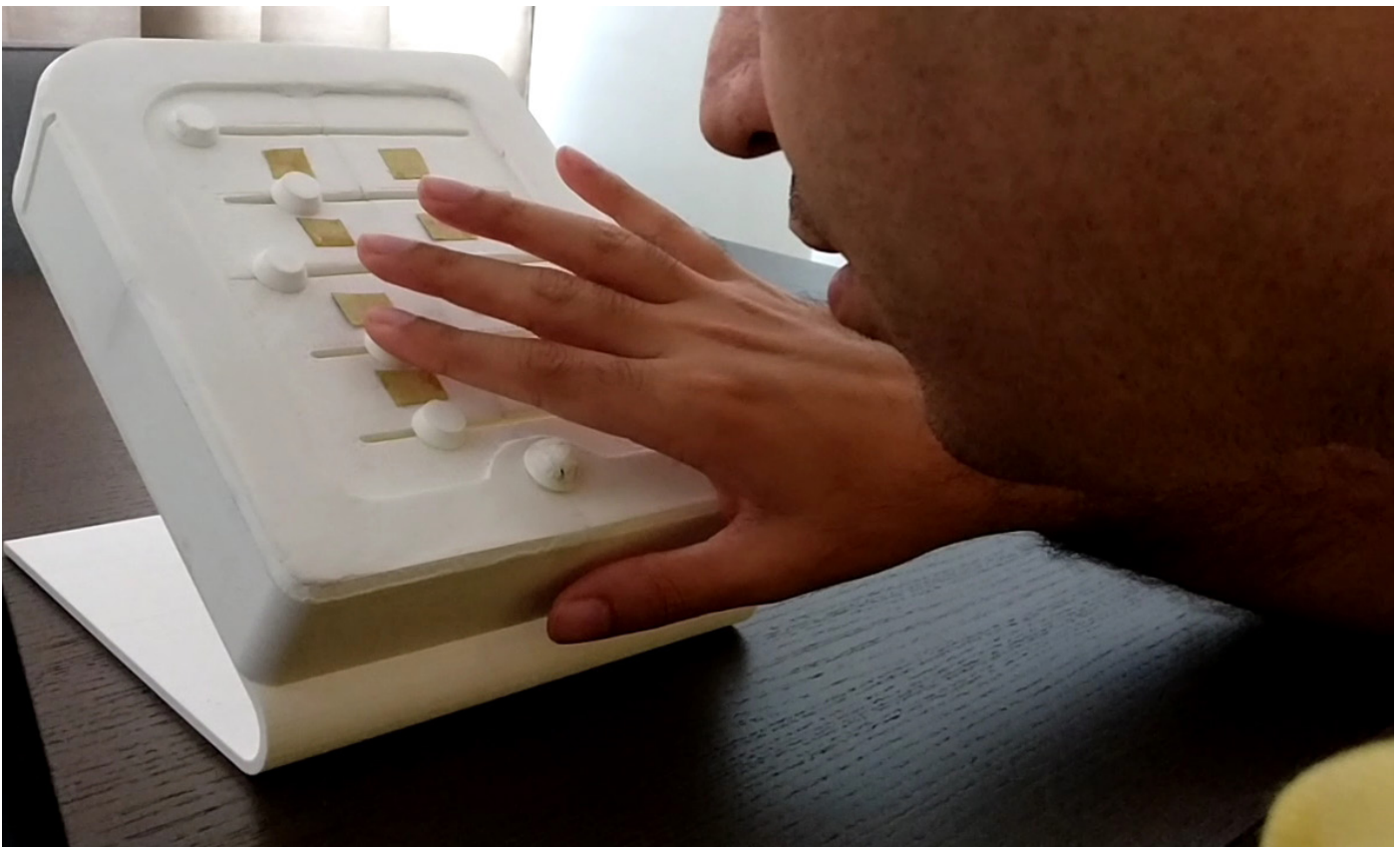
Figure 38 3D printed form prototype presented to a blind programmer, for tactile perception of the product.
