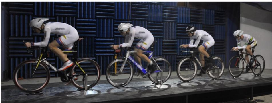
Figure 2.10: Wind tunnel study with four in-line cyclists as conducted by Barry et al. (2015)
