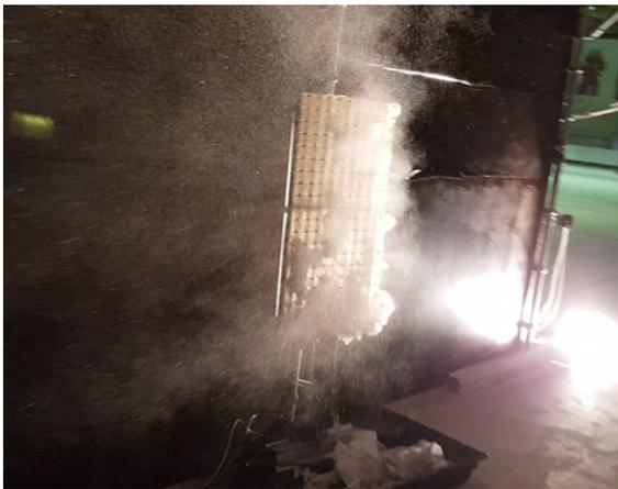
Figure A.1: Bubbles carried downstream immediately after production by seeding rake
