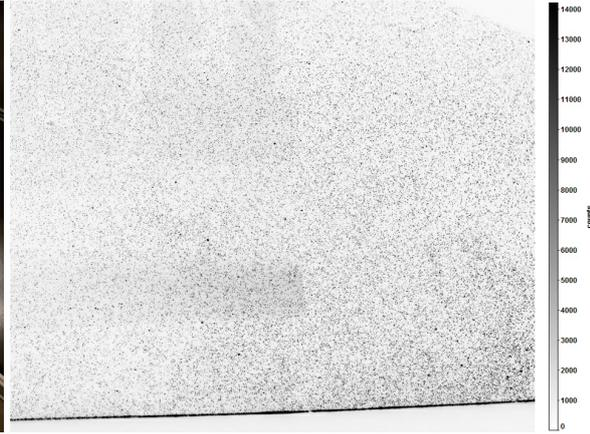
Figure A.4: Improved seeding distribution in measurement plane due to reduced circulation
