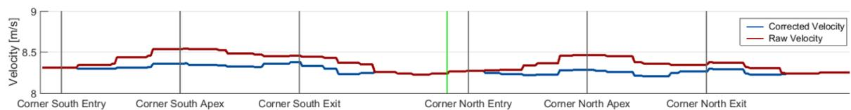
Figure 5.3: Phase-averaged velocity plot using data of individual upright test at  $8.33 \text{ ms}^{-1}$ .
