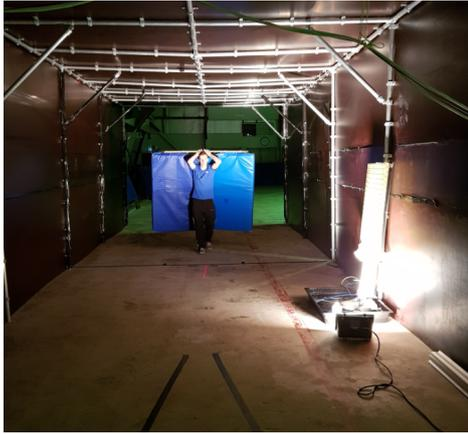
Figure A.3: Mats and later blanket carried by one operator in opposite cycling direction to reduce circulation effect in tunnel
