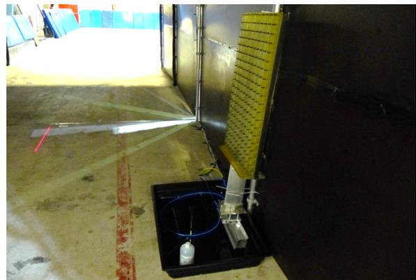
Figure 4.4: Seeding rake attached to vertical tunnel beam standing in a sump
