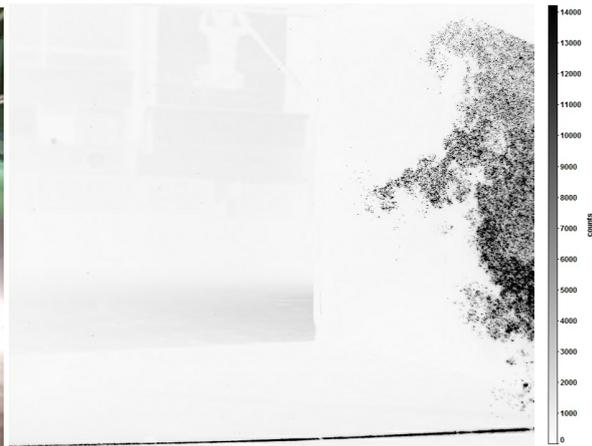
Figure A.2: Initial seeding distribution in measurement plane
