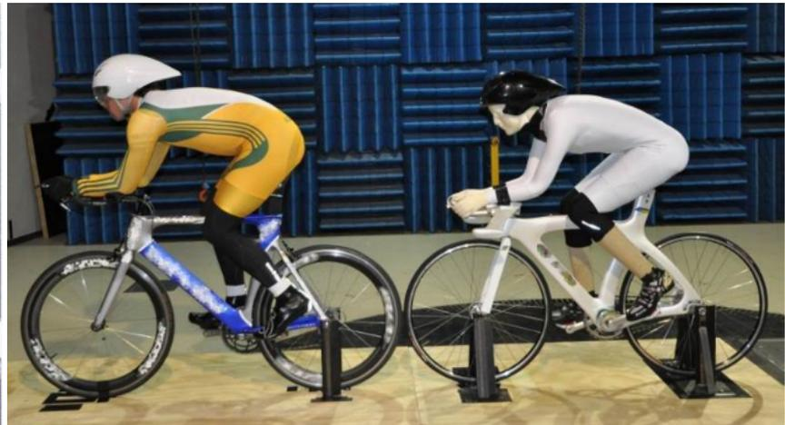
Figure 2.9: Wind tunnel test at minimum separation distance, as conducted in Barry et al. (2014a)
