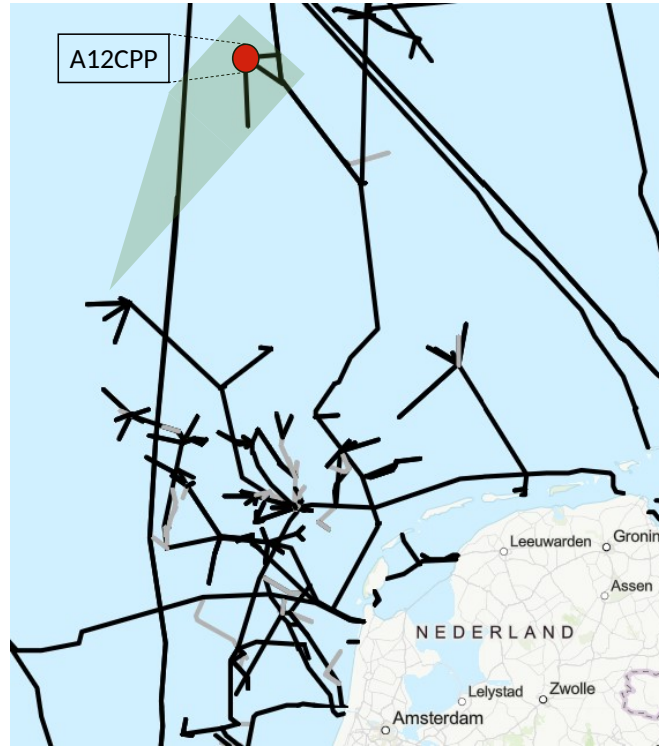
Figure 3.5: The location of the offshore platform and the gas pipeline infrastructure of the North-Sea. The transparent green area represents the Dogger Bank in the Dutch EEZ.
