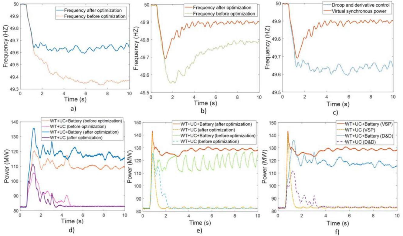
**FIGURE 11.** (a) Frequency of droop and derivative control before and after optimization, (b) Frequency of VSP before and after optimization, (c) Optimized frequency of droop and derivative control and VSP, (d) Power output of droop and derivative control before and after optimization, (e) Power output of VSP before and after optimization, (f) Power output of optimized droop and derivative control and VSP.
