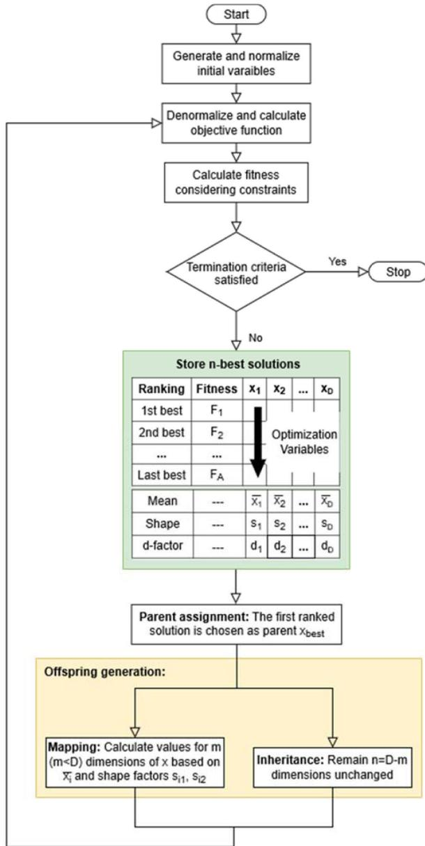
FIGURE 8. The flowchart for the MVMO algorithm procedures.
