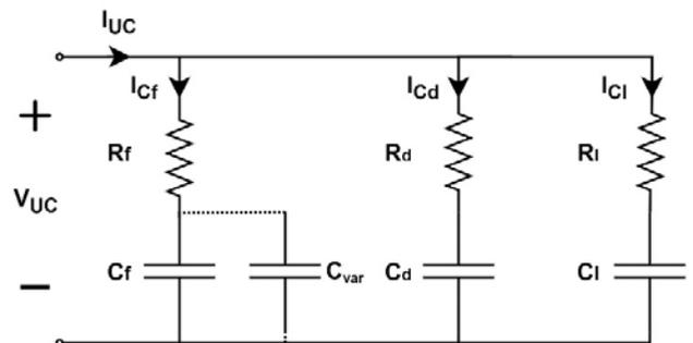
FIGURE 5. Structure of RC parallel branch model.
