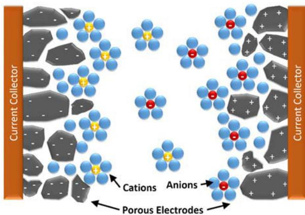
FIGURE 4. Porous structure of an ultracapacitor (inspired by [12]).
