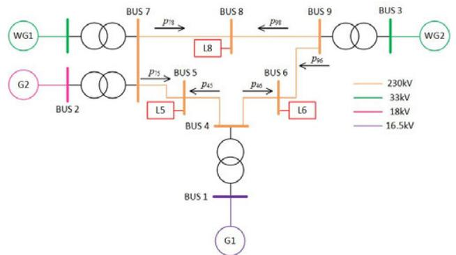
FIGURE 7. IEEE 9 bus system with 52% wind generations.
