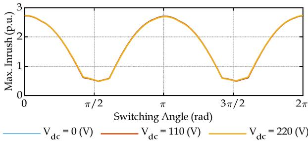
Fig. 7. Effect of switching angle on energization inrush phenomena.
