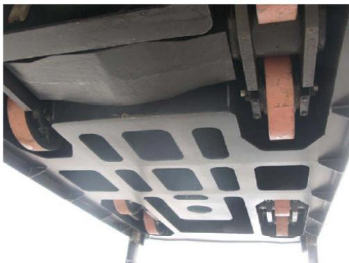
Figure 6.15: A picture of the bottom of the 8-wheel lower roller carriage of the Northern lock in IJmuiden [49]
