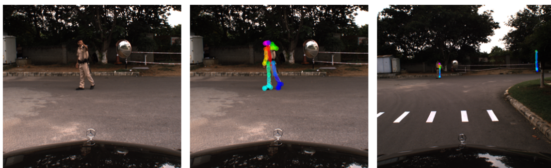
Figure 6.4: Examples of real world skeleton detection using OpenPose. Left image is the input, resulting in the detection of the middle image. Right image shows poor detection and false positives at longer range. Taken from an unlabeled part of GPGD [3]
