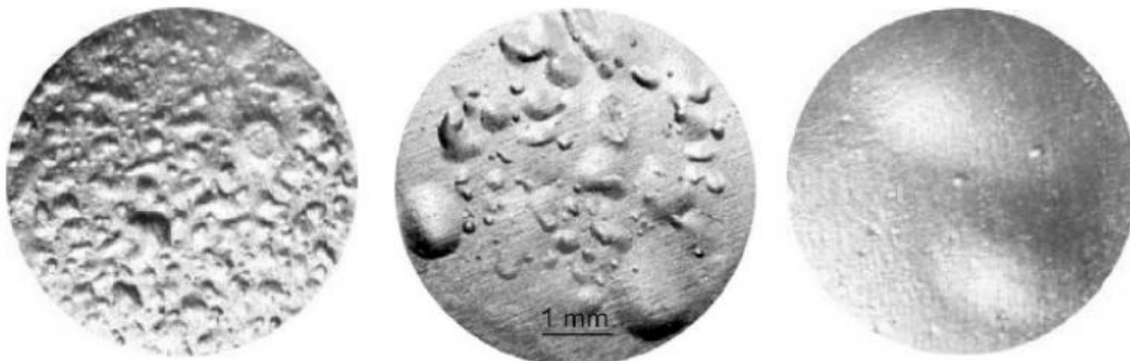
Figure 1.1: Optical micrographs of blisters on the surface of 95% deformed 13Cr2MoNbVB steel after irradiation with hydrogen plasma to 2 \cdot 10^{24} \text{ H/m}^2 at 275 (left), 305 (center) and 323 K (right). The micrographs are made for studying sputtering-induced erosion of plasma-facing materials (PFMs) for future commercial reactors. The scale is the same for all micrographs. [2]
