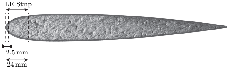
Figure 6.10: Cross-section of the experimental wing.
