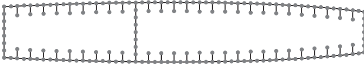
Figure 3.6: Illustration of the cross-sectional discretisation of a wingbox structure including stringers. The dots indicate the cross-sectional nodes.
