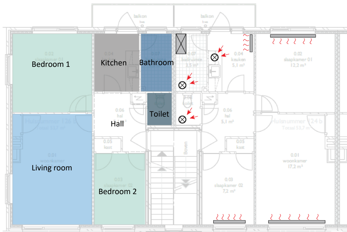
Figure 29: Floor plan Soendalaan with the location of delivery equipment. Adapted from (KAW, 2017, DO-02_b)
