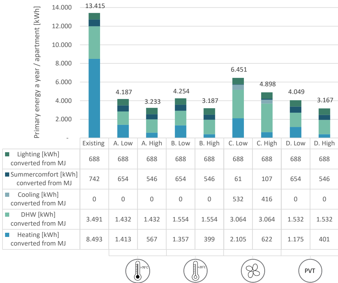
Figure 32: Primary energy consumption per apartment in kWh for all concepts and the existing situation
