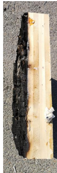
Figure 114: Right CLT panel char depth post testing
