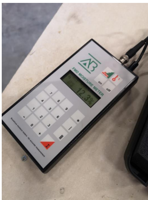
Figure 22: Moisture content sensor being employed before testing a compartment
