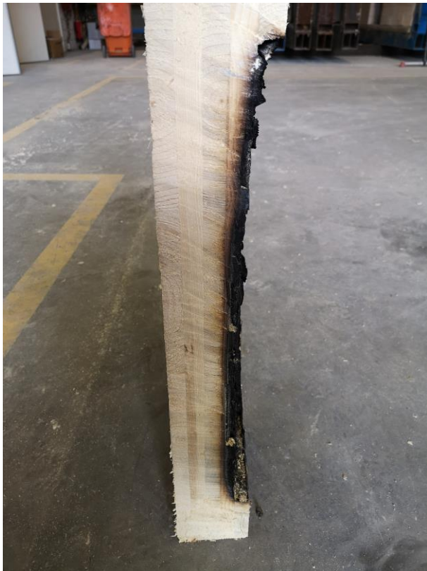
Figure 104: Charring behaviour of the ceiling panel
