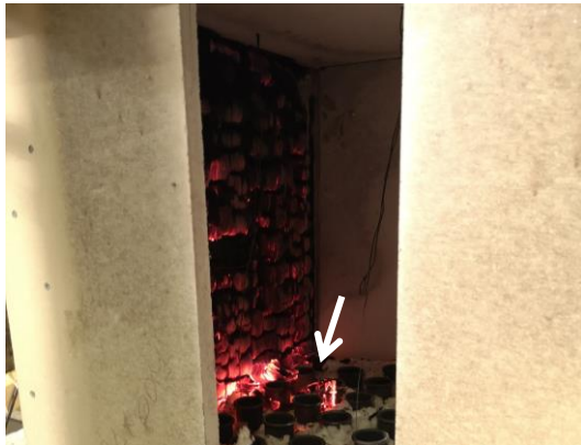
Figure 88: Minor char fall-off observed, as indicated by the accumulation of char on the floor panel (arrow)
