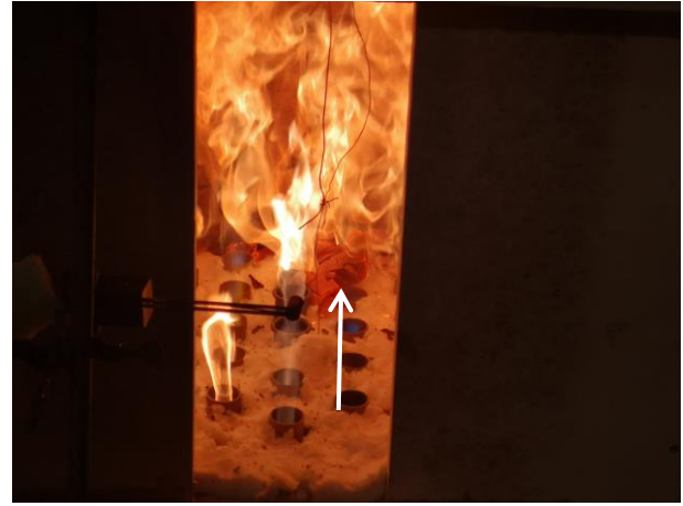
Figure 28: Small char piece that fell off on the floor during the heating phase (as indicated by the white arrow)
