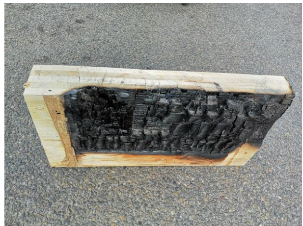
Figure 121: Charring behaviour of the ceiling panel
