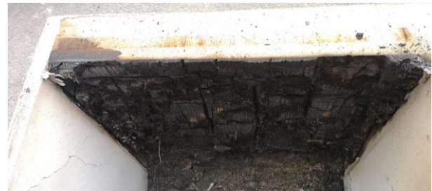
Figure 81: Charring depth after the experiment on the right wall
