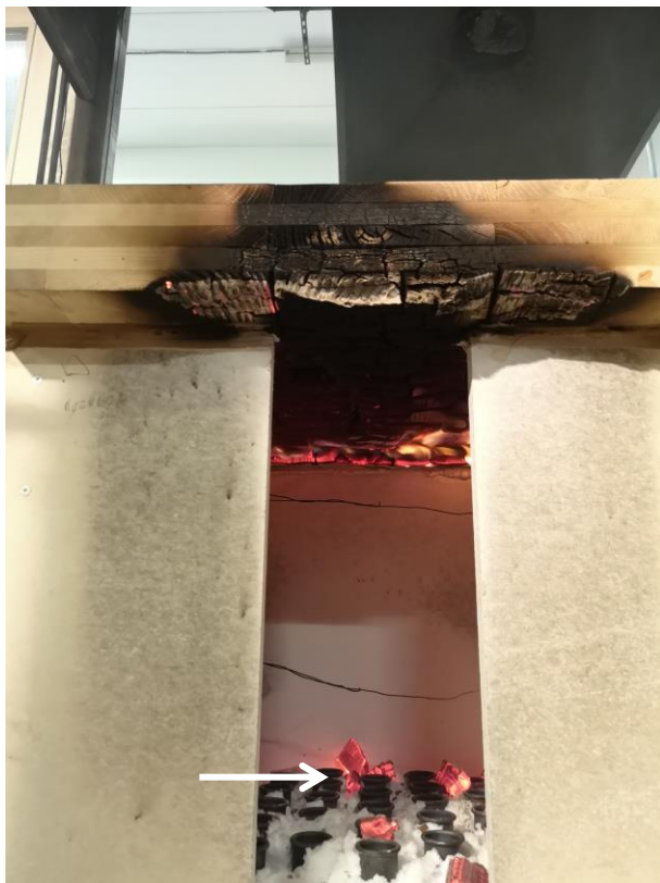
Figure 120: Minor char fall-off during MUF- C-2
