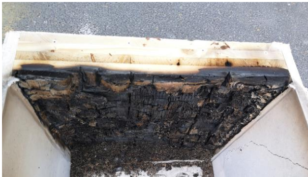
Figure 80: Charring depth after the experiment on the left wall
