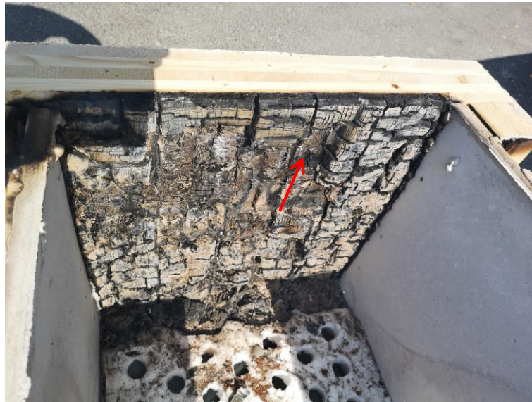
Figure 29: Charring depths post testing with arrow indicating locations of visible char fall-off
