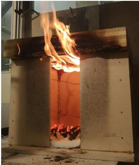
Figure 97: Additional charring at the ventilation opening post burner switch-off
