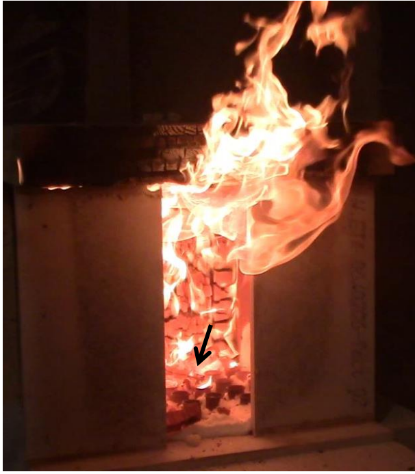
Figure 102: CLT panels at the instant the burner bed was switched off. Char Fall-Off during the heating phase indicated by the black arrow
