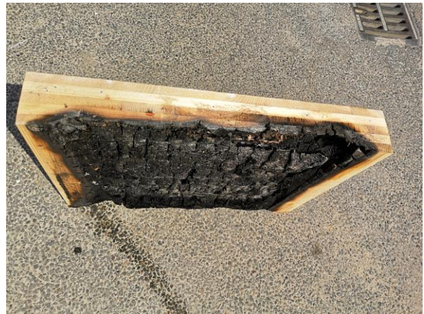
Figure 105: Charring behaviour of the back panel
