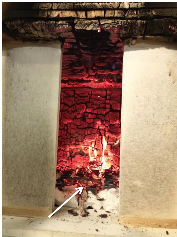
Figure 126: Evidence of local char fall-off as indicated by accumulated char on the floor panel
