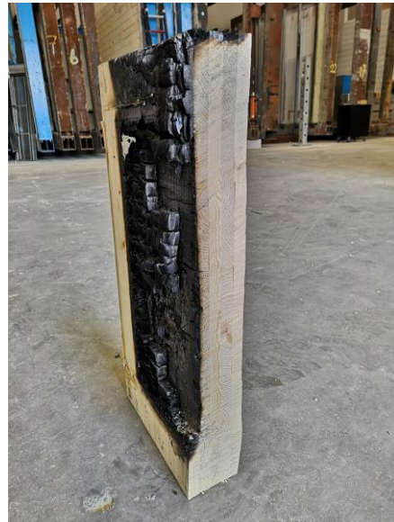
Figure 98: Charring depth of the ceiling panel
