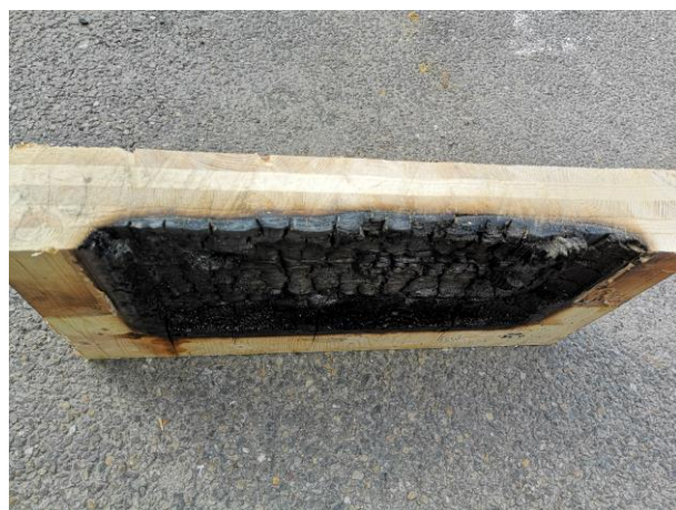
Figure 128: Charring behaviour of the Ceiling Panel
