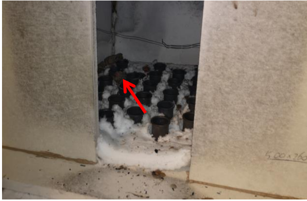
Figure 95: Minor pieces of char that fell off as indicated by the arrow
