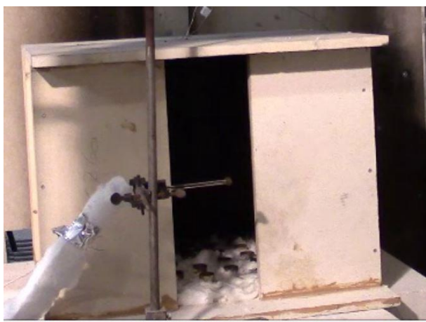
Figure 25: CLT back wall before reignition of the burner bed
