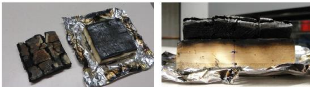
Figure 36: Debonded PU bonded CLT sample, from Crielaard (2015)
