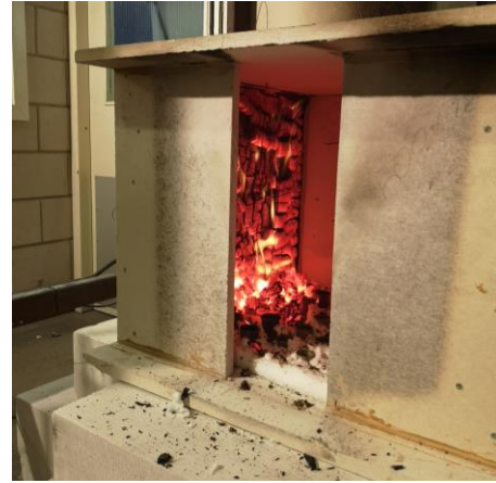
Figure 79: Evidence of local char fall-off from the left side wall. Picture taken after a period where char segments broke-off gradually.
