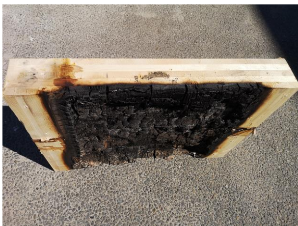
Figure 127: Charring behaviour of the back panel
