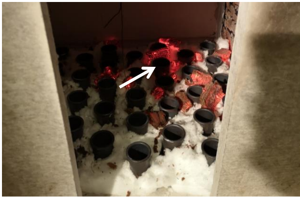
Figure 113: Small pieces of fallen off char as indicated by the white arrow
