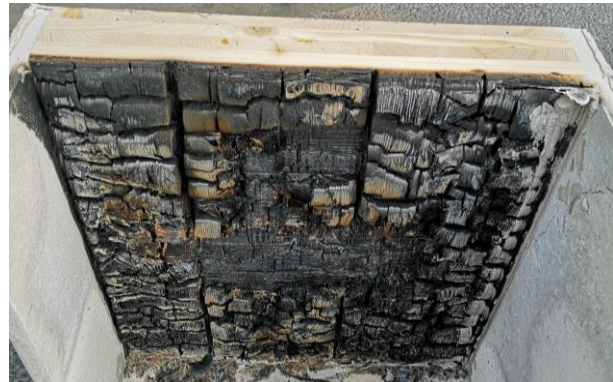
Figure 89: Left CLT panel char depth
