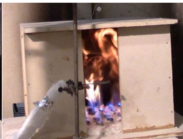
Figure 26: CLT again entering flaming combustion
