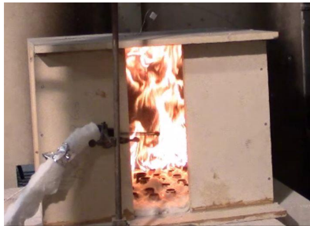
Figure 24: CLT back wall at the moment of burner outage
