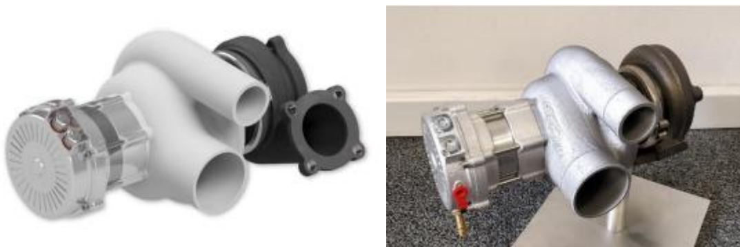
FIGURE 2.4– FIGURES OF THE SECOND MOCK-UP OF THE ELECTRIC ASSISTED TURBOCHARGER. IN THIS DESIGN, A COMPRESSOR HOUSING IS DESIGNED WHERE THE DONUT SHAPED ATTACHMENT IS INCORPORATED IN THE COMPRESSOR HOUSING [4].
