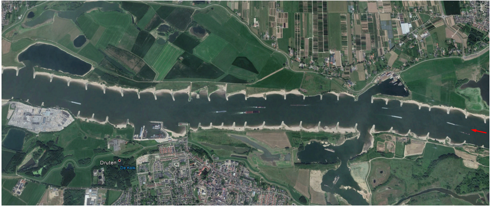
Figure 1.1: Examples of traditional river training with transverse groynes. Waal River near Druten, The Netherlands. Source: Google Earth © 2017. Red arrow indicates flow direction.
