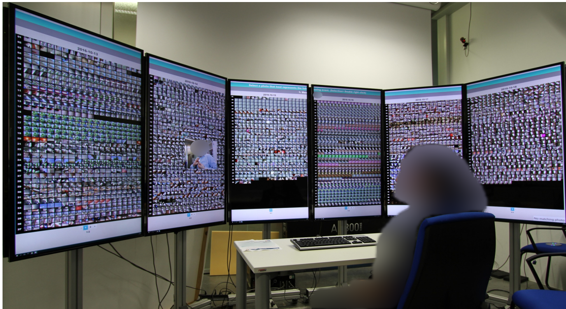
Figure 1: “Pixel Memories”: A lifelog visualization prototype consisting of six 50-inch screens, each presenting a day in the life of a participant. Each entry in the grid is a photo captured every 30 seconds automatically by a clip-on camera. The screens show a maximum of 4218 photos at a glance (703 photos per screen).
