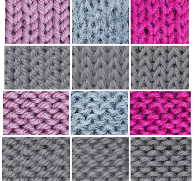
Fig. 9. 1st and 3rd rows: images of a real knitted cloth (made with yarns from the top row of Fig. 10) for the pattern consisting of knit (1st row) and purl (3rd row) stitches. 2nd and 4th rows: rendering of the same stitch pattern with the inferred yarn with default material settings.
