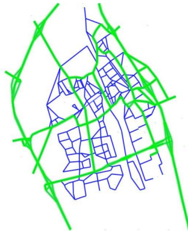
FIGURE 1 AD Subnetwork: feasible links for AD subnetwork are shown with (bright) green and the rest with (dark) blue.
